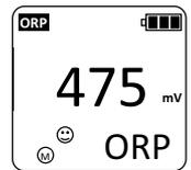
**Note:** This procedure allows user to adjust reading upwards only. If displayed reading during calibration is higher than reference value (490 mV in 475 mV calibration solution) keep pressing **MODE** until required value is achieved (taking into account that max adjustment is -75 mV).
