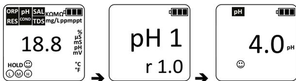
All segments ON -> model name + software release -> measurement
